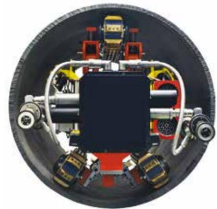
Diakont's RODIS tethered robotic EMAT tool was used to complete a direct assessment casing inspection delayed by changed permit conditions. NT ILI was deployed and completed the project six days after initiation by inserting the tool outside the disputed permit area and coordinating the outage with a nearby replacement project.
