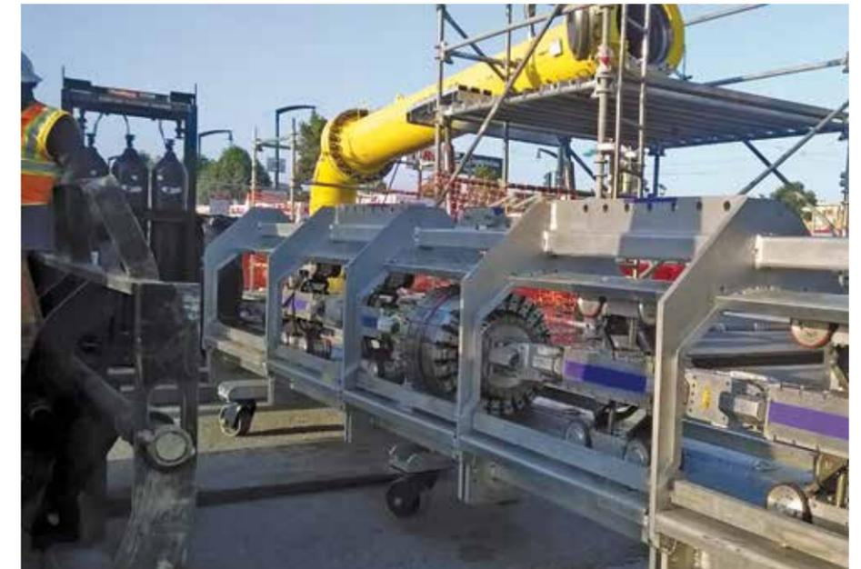
Pipetel's Explorer untethered robotic MFL tool ready for deployment into pressurised pipeline as part of a project to inspect multiple inserted pipe segments in a major metropolitan area.
