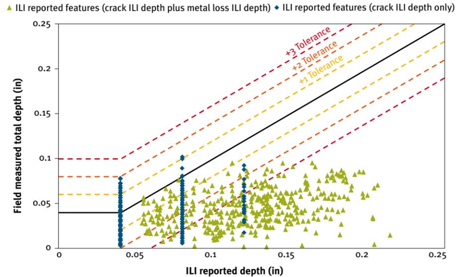
Figure 6: Feature depths (with and without metal loss ILI depth included).
